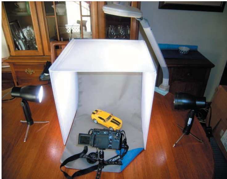
This is a photo box I bought from Micro-Mark called the "Photo Studio in a Box" (Part #84628) and it is what I use 90% of the time to do my photos for Model Car Builder magazine. It sells for less than $100.00 and includes the light box, two lights, a camera holder, backdrop, & carrying case (no camera).
