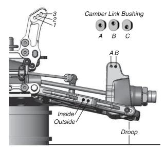
*Oil:* 35wt Spring: Blue Piston: Stock Limiters: \_0\_\_\_\_\_ Sway Bar: B Camber: <u>-2.0</u> **Toe:** -1.0 Camber Link Bushing: C, Lower Outer Camber Link: B Caster Block: 10° Ackerman Placement: Middle Upper Shock Placement: 2 Lower Shock Placement: Inside Droop: 38mm Ride Height: 27mm Bump Steer Spacers: 3 Washers on the Steering Knuckle
