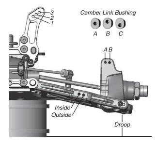
*Oil:* 35wt Spring: Black Piston: Stock Limiters: 0 Sway Bar: C **Camber:** <u>-2.5</u> **Toe:** -1.0 Camber Link Bushing: B, Upper Outer Camber Link: B Caster Block: 10° Ackerman Placement: Middle Upper Shock Placement: 2 Lower Shock Placement: Inside Droop: 34mm Ride Height: 27mm Bump Steer Spacers: 3 Washers on the Steering Knuckle
