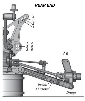
**Oil:** 30wt Spring: Black Piston: Stock Limiters: 0 Sway Bar: B Camber: <u>-2.0</u> Inner Camber Link: 3 Outer Camber Link: A **Rear Toe-In:** 3° (Optional) Rear Anti-Squat: 3° (Optional) Hub Carrier Placement: Down and Forward Upper Shock Placement: 3 Lower Shock Placement: Inside Droop: 19mm Ride Height: 26mm Wing Position: Upper
