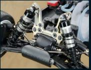
Behind the front humper, the aluminum suspension arm pivot has setscrews to hold the pins in place. The screw pins have hex heads on one side and locknuts on the other.
