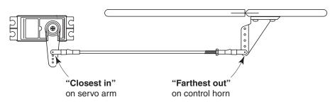
will increase the servo's centering capabilities and output torque, minimize any free play in the system and allow high ATV settings for optimum servo resolution and positive control "feel." **Note:** When the pushrod is "close in" on the servo arm, make certain the servo arm can travel through its full range of movement without the pushrod (or clevis or other type of connector) interfering with the servo arm, output shaft or servo case.
