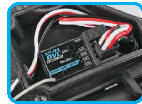
DVC (Dynamic Vehicle Control) receiver with built-in gyro.
