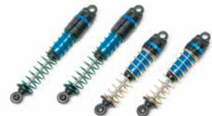
Blue anodized aluminum V2 coil-over shocks
