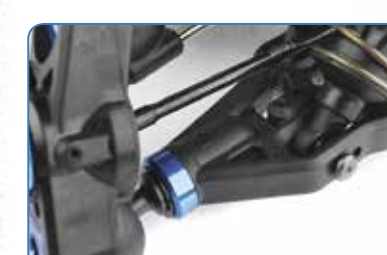
94mm CVA driveshafts increase traction and chassis support
