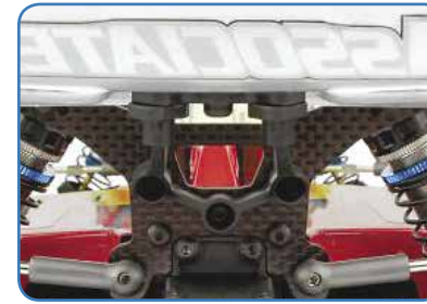
Stiff, lightweight 4mm thick carbon fiber shock towers
