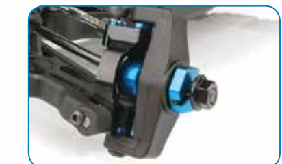
12mm aluminum drive hexes both front and rear
