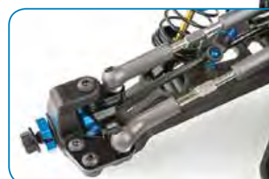
Robust suspension arms with multiple shock mounting positions
