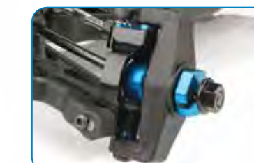
12mm aluminum drive hexes both front and rear
