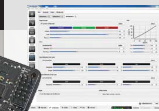
The CC3D flight controller is pre-programmed using LibrePilot.
