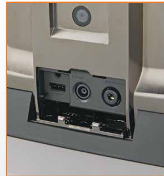
Update and program S.Bus servos using the built-in S.Bus port.
