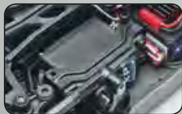
XP metal-gear steering servo
