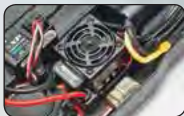
Water-resistant Reedy SC600-BL sensorless brushless speed control
