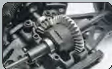
Front and rear sealed metal gear differentials and tough aluminum drive shaft
