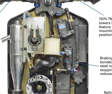
7075-T6 aluminum shock towers front and rear feature finely tuned shock mounting upper arm positions.
