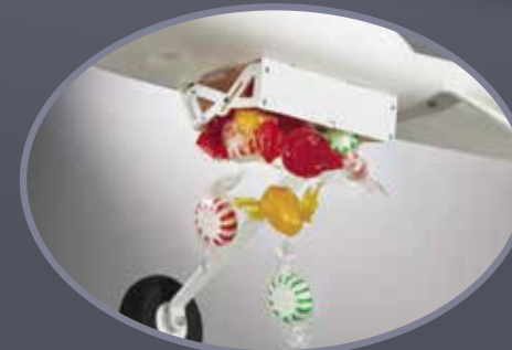
Operate the "drop-door" from the 5th channel of your radio for in-flight deployment of a parachute or other creative payloads!
