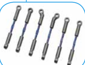
Heavy-duty ball cups and ball studs allow for maximum suspension travel while reducing binding and friction
