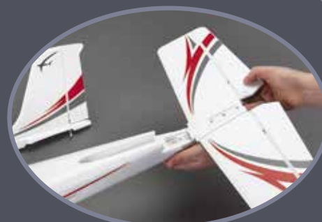
The tail section aligns itself automatically and is secured with just one screw.
