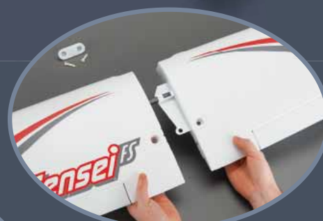
The wing halves slide together onto a tube and are secured with two bolts.
