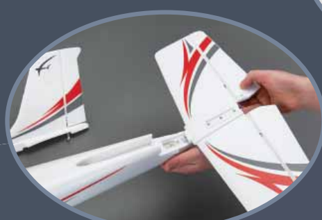
The tail section aligns itself automatically and is secured with just one screw.
