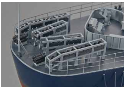
The rear of the boat features mine laying racks and anti-aircraft guns.
