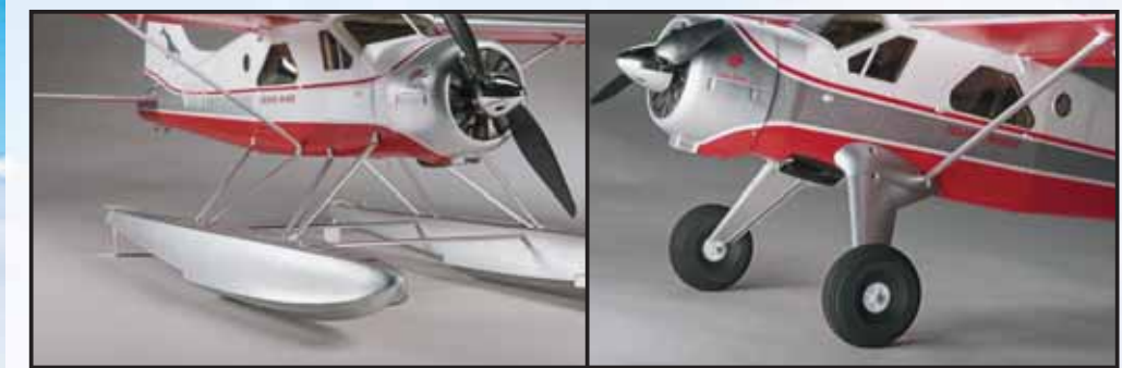
Water rudders on the floats provide control for water takeoffs and landings. The conventional landing gear comes with big, tundra-style tires.
