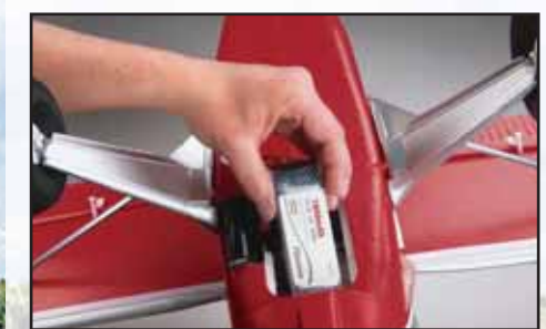
A hatch on the bottom of the fuselage provides easy access to the battery compartment. Battery shown not included.
