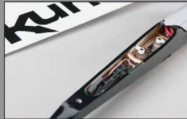
A micro receiver and two micro servos fit neatly inside the fiberglass fuselage.
