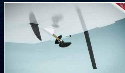
The FRP prop is offset to maximize performance. The center-mounted skeg helps keep the boat under control through turns.
