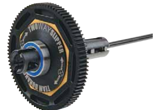
Two-way center slipper for more adjustability and power stabilization.
