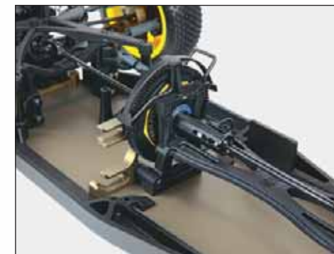
Center UJ drive shafts front and rear for increased efficiency and drivetrain smoothness.
