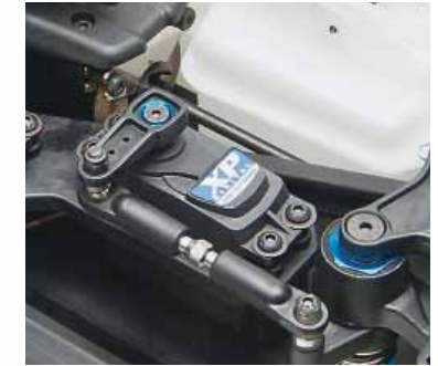
High-torque XP DS1510MG metal gear steering servo.
