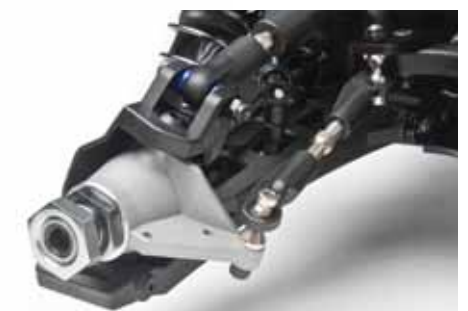
Aluminum steering knuckles for improved durability.
