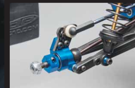
Factory Team 7075-T6 blue aluminum 0° rear hubs with oversized outer bearing and 12mm hex drives.
