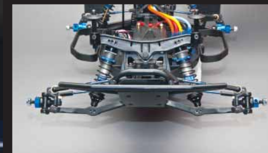
"Gull-wing" front suspension arms and updated shock towers optimized for Big Bore shocks.
