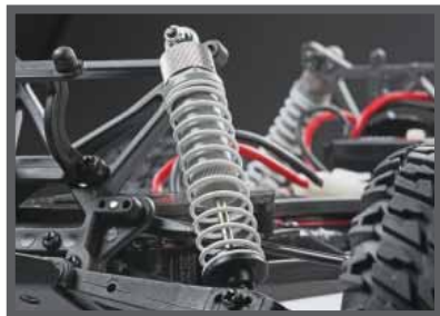
Oil filled shocks with metal caps.
