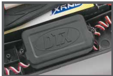
Waterproof receiver box and steering servo.
