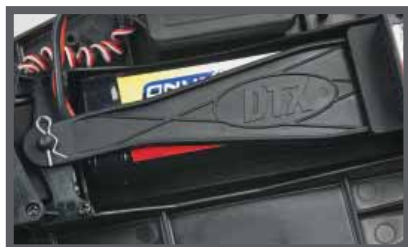
Compatible with 6-7 cell NiCd/NiMH and 2S hard case LiPo batteries.
