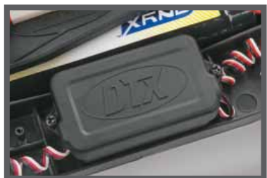
Waterproof receiver box and steering servo.
