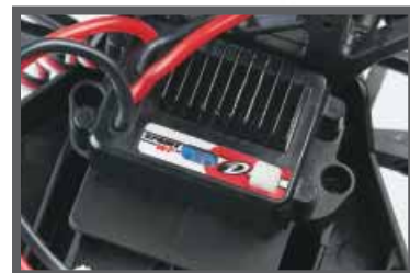
Waterproof ESC with brake, reverse and battery cut-off.
