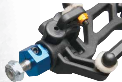
Factory Team 12mm blue aluminum front and rear clamping hexes with hex wheels
