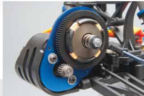
VTS slipper assembly featuring high-resolution spring
