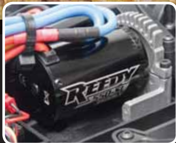
Brushless Reedy 550-SL 3500kV motor
