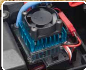
Water-resistant XP speed control with Deans® Ultra Plug® battery connector
