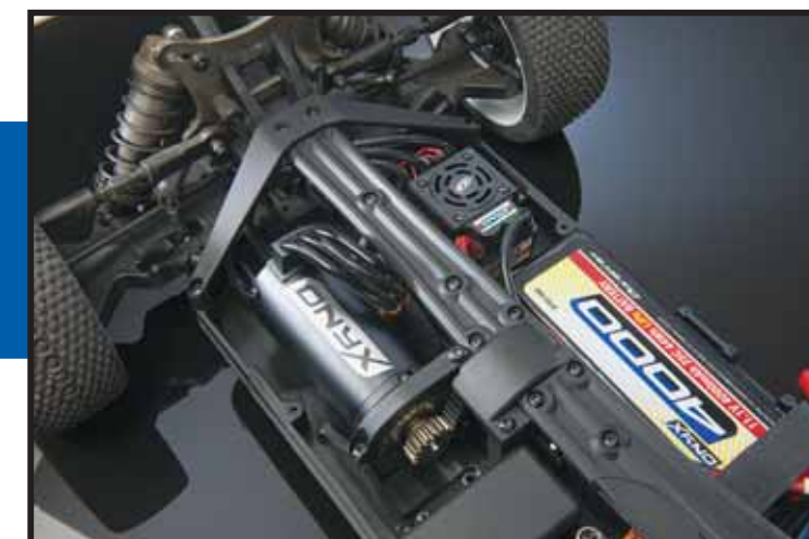
DTXC3194 Onyx 1/8 Scale Brushless System 2200kV DTXC3195 Onyx 1/8 Scale Brushless System 2650kV
