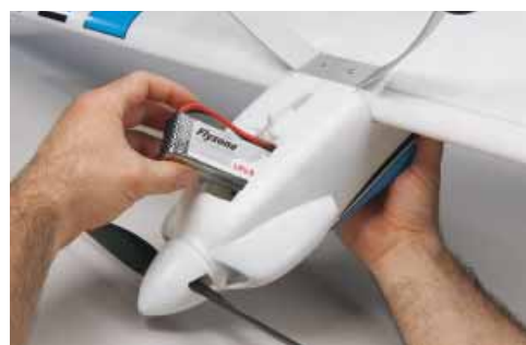
Easy access to the battery is provided through this hatch.
