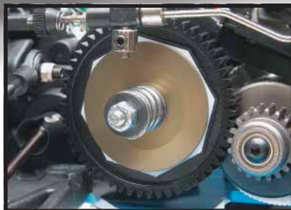
V2 dual disc slipper clutch with low center of gravity of transmission
