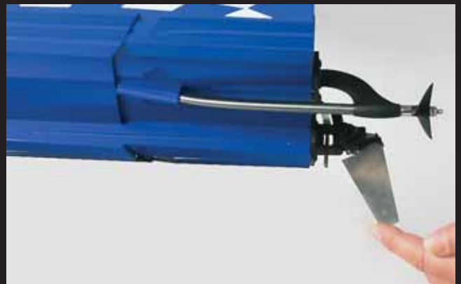
The rudder flexes upon impact to limit damage.
