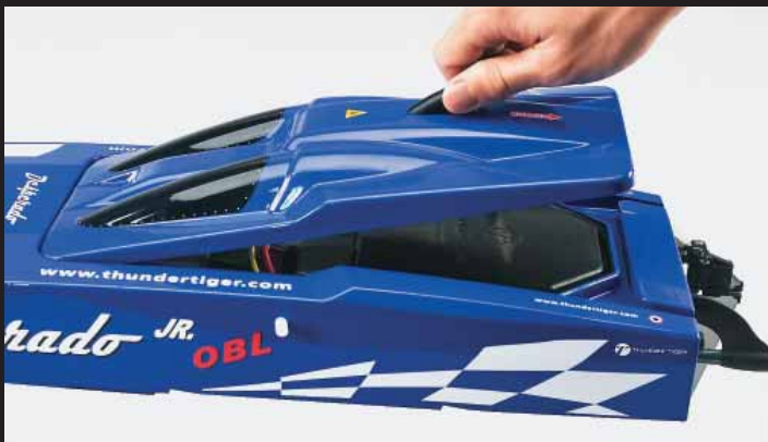
A magnetic hatch makes for quick and easy access to on-board gear.
