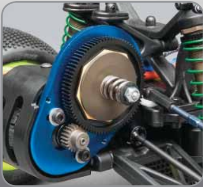
V2 slipper clutch with high-rate spring for finer adjustment increments.
