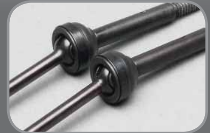
CVA joints with pin retainer clips.
