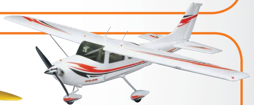
Select Scale Cessna® 182 Skylane® Legendary style Wingspan: 47.5 in (1205 mm) Weight: 2.3 lb (1050 g) HCAA2520
