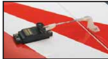
Servos on each wing panel maximize mixing options, while simplifying set-up.
