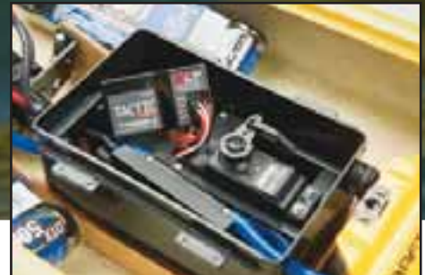
The compact receiver, servo and water-cooled, brushless 45A ESC are installed inside a watertight box.
