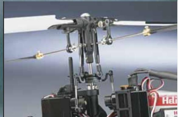
With its collective-pitch rotor head and the swift, precise response of Bell-Hiller mixing, the Novus 125 CP is fully aerobatic and 3D capable.
