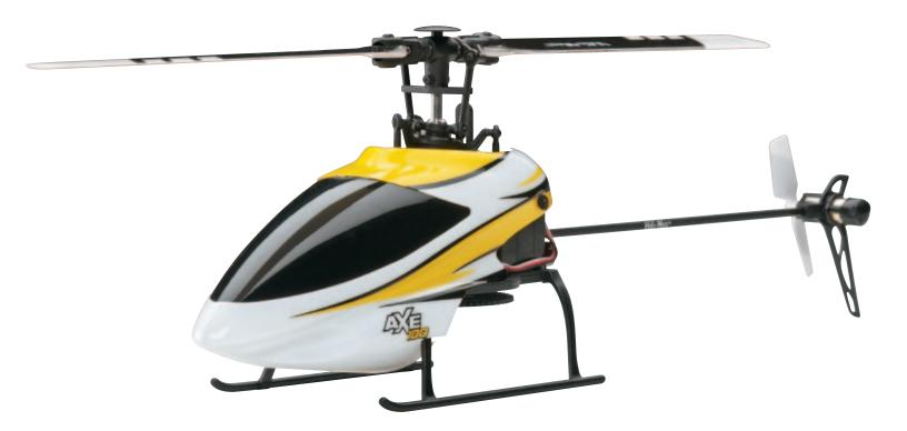
The features that make the Axe 100 CP a superior aerobat are also the ones that make it one of the most innovative helis available. A flybarless collective pitch head gives it a wide performance range, making it easy to maneuver and control in the smallest of spaces. The "TAGS" triple-axis gyro adds confidence-building stability. Both the RTF and Tx-R versions feature SLT compatibility, and include two LiPo flight packs, a charger, spare blades, linkages and a screwdriver.
