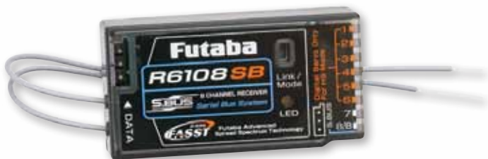
R6108SB 8-Channel Programmable Air Dimensions: 1-7/8 x 1 x 9/16 in (47 x 25 x 14 mm) Weight: 0.5 oz (14.0 g); Weight w/o case: 0.33 oz (9.3 g) FUTL7660
