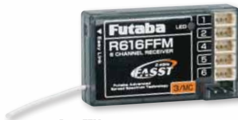
R616FFM 6-Channel Micro Park Flyer (Micro Connector) Dimensions: 1-9/16 x 7/8 x 5/16 in (39 x 23 x 8 mm) Weight: 0.22 oz (6.3 g); Weight w/o case: 0.14 oz (4.0 g) FUTL7626
