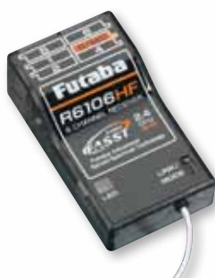
R6106HF 6-Channel Park Flyer Dimensions: 1-1/2 x 7/8 x 1/2 in (39 x 22 x 12 mm) Weight: 0.3 oz (6.9 g) FUTL7650
