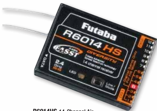
R6014HS 14-Channel Air Dimensions: 2-1/2 x 1-1/2 x 5/8 in (52 x 38 x 16 mm) Weight: 0.8 oz (22.0 g) FUTL7645
