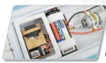
Lift off the cowl, and you'll see that all components are positioned for easy access and maintenance. The Rio EP accepts both 6-cell stick and 7-cell hump battery packs.
