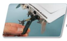
If the Minimono strikes an object in the water, a breakaway feature allows the rudder to swing back and avoid damage. It quickly snaps back into place.
