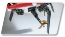
The surface drive system effectively delivers power with low maintenance. The included GrimRacer metal prop maximizes the Zenoah G260PUM engine's high output.
